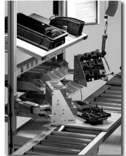
Manual Assembly Station
