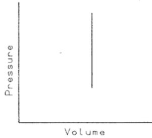
Fig. 2.3 Constant volume, non-flow process
