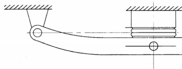
Fig. 5.4 Suspension arm with bellows air spring
