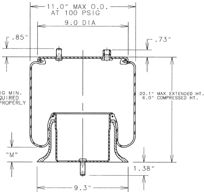
NOTE: 10 PSIG MIN. PRESSURE REQUIRED TO OPERATE PROPERLY
