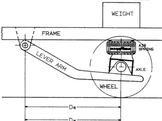
$f_s = f_n / \sqrt{L_r}$  The natural frequency of the suspension is also dependent on the placement of the air spring in relation to the axle (lever arm ratio). Given a load and design height, one can look up the spring's natural frequency (in the Dynamic Characteristics Table in the Engineering Data Section) and see how the location of the spring would affect the suspension's natural frequency:
