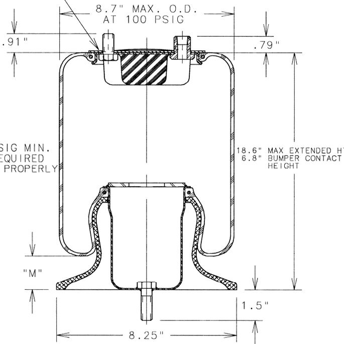
NOTE: 10 PSIG MIN. PRESSURE REQUIRED TO OPERATE PROPERLY
