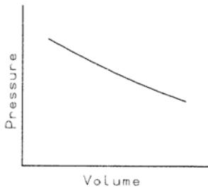
Fig. 2.4 Constant temperature non-flow process (isothermal process)
