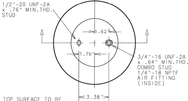
TOP SURFACE TO BE FULLY SUPPORTED BY 7.7" DIA. PLATE
