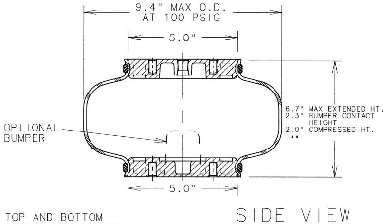
TOP AND BOTTOM SURFACE TO BE FULLY SUPPORTED BY 9.65" DIA. PLATE OR SEE INSTALLATION GUIDELINES SECTION FOR ALTERNATE MOUNTING OPTIONS
