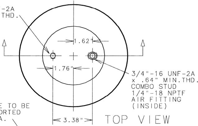
TOP SURFACE TO BE FULLY SUPPORTED BY 7.7" DIA. PLATE
