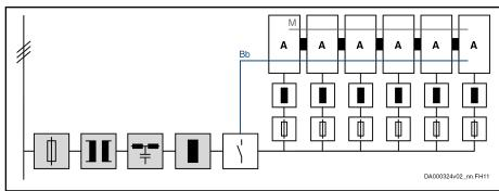
Components marked with gray background color: Optional, depending on the application; the choke is used to reduce current harmonics Component HCS01 (all components A identical); connected to supply
