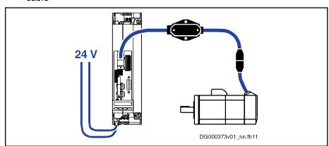
Fig.8-13: Control Voltage Switched On and Encoder Connected
