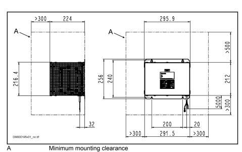
Fig.8-46: Dimensions (with Suspended Mounting on the Wall)
