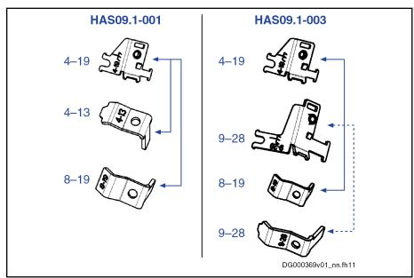
HAS09.1-0 Plates for cable diameters 4-13 mm and 8-19 mm 01
