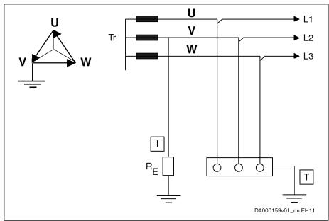
Isolation of all active parts from ground, connection of one phase - generally phase V - to ground or via an impedance  $R_{\text{E}}$ 1 =
