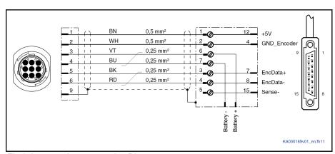
Fig.8-21: Interconnection Diagram
