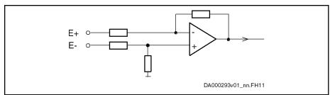
Fig.7-17: Input Circuit for Resolver Evaluation (Block Diagram)
