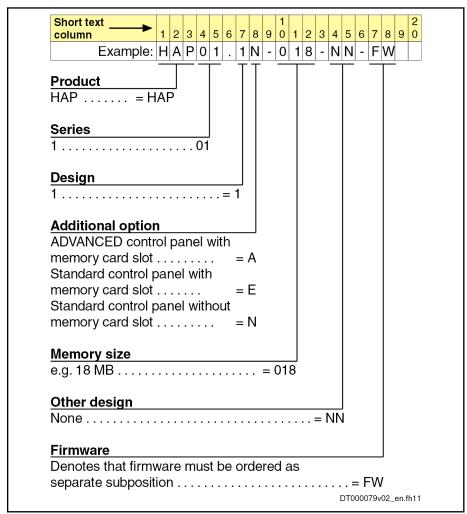
Fig.1-4: Type Code of Control Panel
