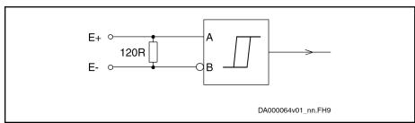
Fig.7-18: Input Circuit for Square-Wave Signals (Block Diagram)
