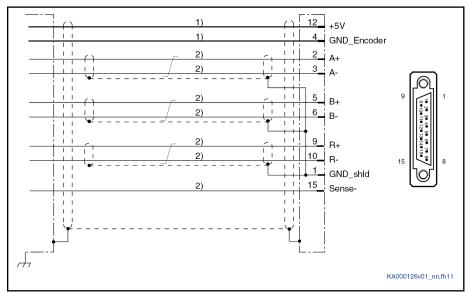
1) Line cross section ≥ 0.5 mm<sup>2</sup>; observe allowed encoder cable length 2)
