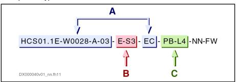
A Basic device (maximum current [W0028 = 28 A], line [03], on-board connection point [EC])
