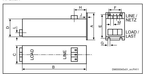
Type NFE02.1-230-008 (with 3 terminal connectors) Fig.8-39: Single-Phase Filter NFE02.1 for Drives
