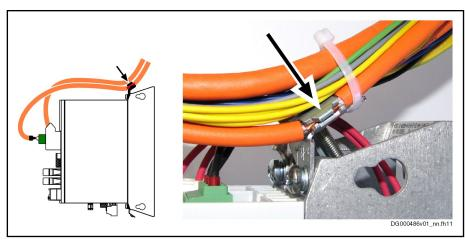
Fig.6-13: Shield Connection of Shielded Lines at the Top of the Device
