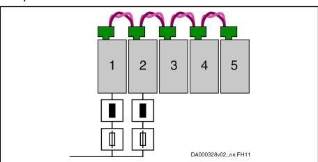
1, 2 HCS01.1E-W0028 (supplying devices) 3, 4, 5 HCS01.1E-W0018 (supplied devices)
