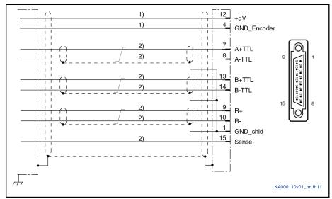
1) Line cross section ≥ 0.5 mm²; observe allowed encoder cable length
