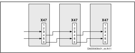
Fig.4-37: Looping through the Module Bus
