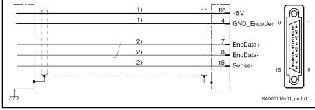
Line cross section ≥ 0.5 mm²; observe allowed encoder cable length
