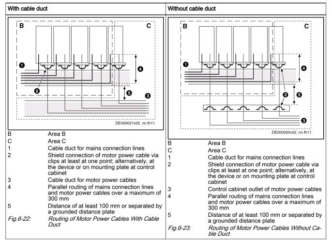
Tab.6-34: Routing of Cables for Converter
