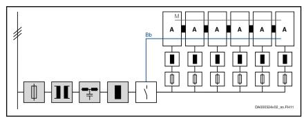
Components marked with gray background color: Optional, depending on the application; the choke is used to reduce current harmonics
