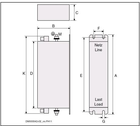
Fig.8-40: Three-Phase Current Filter NFD03.1 for Drives
