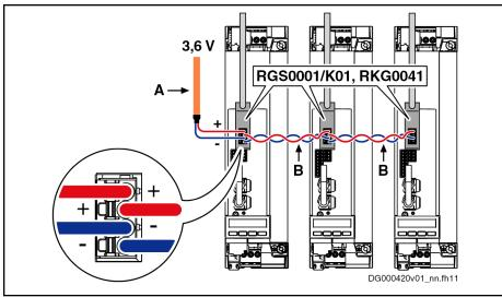
3.6 V Direct voltage source (battery or UPS)
