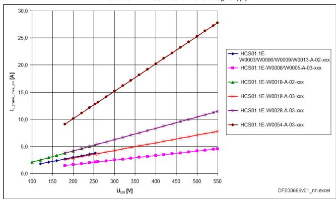
$\begin{array}{ll} I_{L\_trans\_max\_on} & \quad \text{Maximum inrush current} \\ U_{LN} & \quad \text{Mains Voltage} \end{array}$
