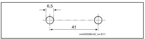
Fig.8-9: Boring Diagram for Battery Box
