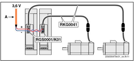
3.6 V Direct voltage source (battery or UPS)
