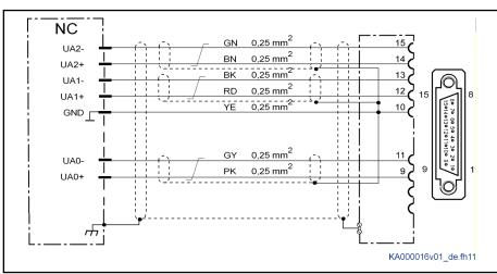
Fig.7-19: Connection of Incremental Actual Position Value Output
