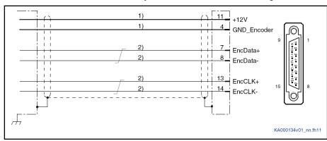
1) Line cross section ≥ 0.5 mm²; observe allowed encoder cable length
