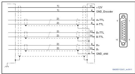
1) Line cross section ≥ 0.5 mm²; observe allowed encoder cable length
