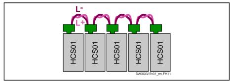
Fig.4-34: Looping Through via DC Bus Connector
