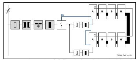
Components marked with gray background color: Optional, depending on the application; the choke is used to reduce current harmonics
