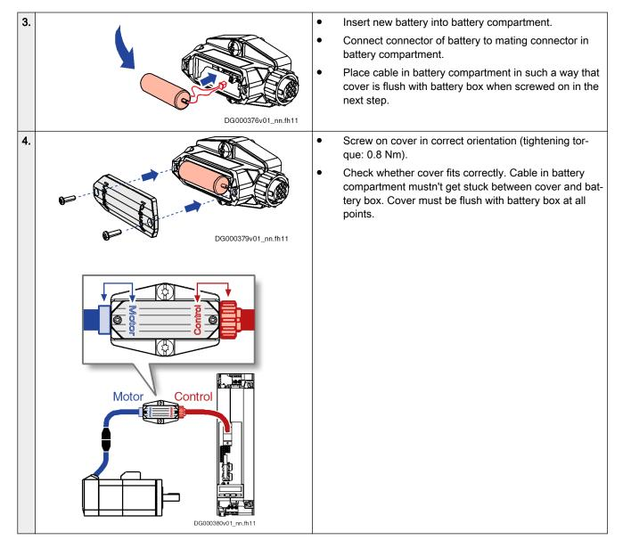
Tab.8-7: Replacing the Battery
