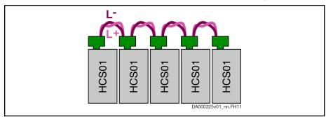
Connecting the DC Buses via DC Bus Connectors Fig.8-5:
