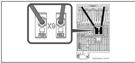
Fig.6-8: Connecting the Braking Resistor (HCS01.1E-W0054)
