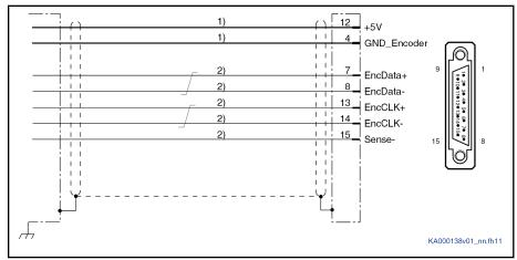
Line cross section ≥ 0.5 mm<sup>2</sup>; observe allowed encoder cable length 1)
