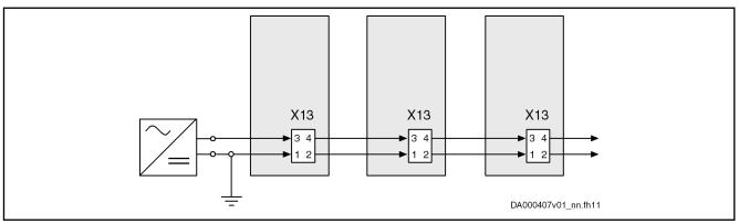
Fig.4-15: Looping Through the Control Voltage
