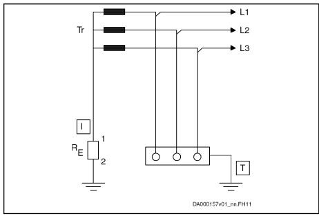
Isolation of all active parts from ground or connection of one point to ground via an impedance RE
