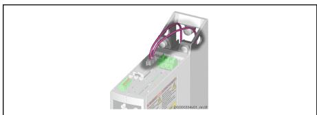
Fig.6-7: Connecting the Braking Resistor (HCS01.1E-W0003...W0028)
