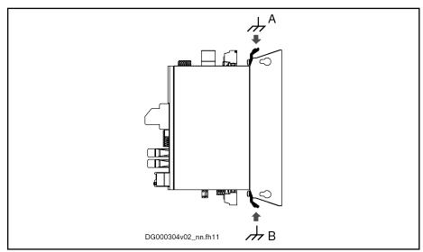
A Shield connection control lines B Shield connection motor cable
