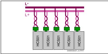
DC Bus Connection via Connecting Bar Fig.4-36:
