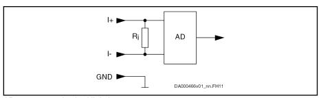
AD Analog/digital converter Fig.7-35: Analog Current Input
