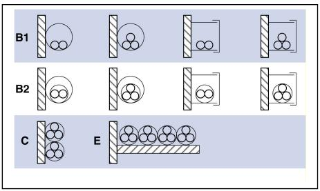
B1 Conductor in installation pipes and in installation channels to be
