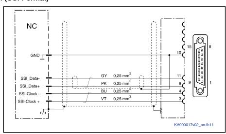
Fig. 7-23: Output of Absolute Actual Position Values According to SSI Format
