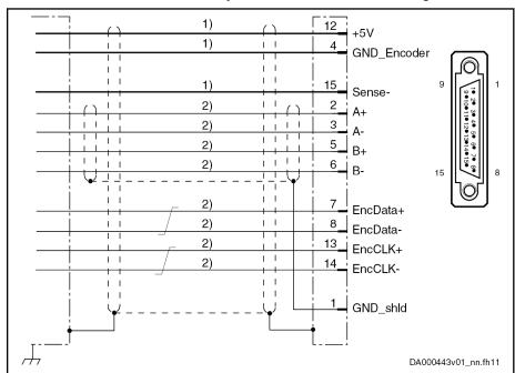
1) Line cross section ≥ 0.5 mm²; observe allowed encoder cable length
