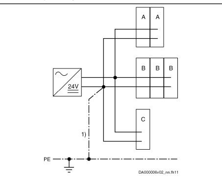
A Number of devices is limited to 2 components with a current consumption of ≤ 5 A / component
