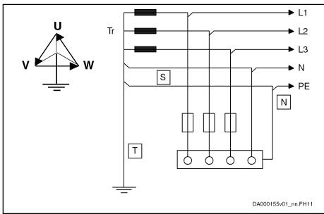
T = Direct grounding of a point (station ground)
