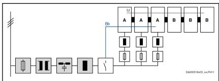
Components marked with gray background color: Optional, depending on the application; the choke is used to reduce current
