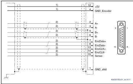
Line cross section ≥ 0.5 mm²; observe allowed encoder cable length
