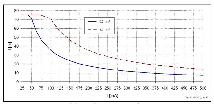
I [mA] I [m] 0.5 mm<sup>2</sup>; 1.0 mm<sup>2</sup> Encoder current consumption
