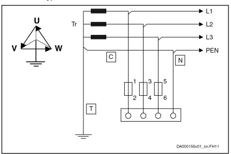
Direct grounding of a point (station ground)
