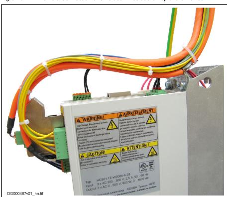
Fig.8-17: Example of a Complete Wiring
