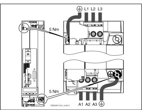
L1, L2, L3 Mains connection A1, A2, A3 Motor connection
