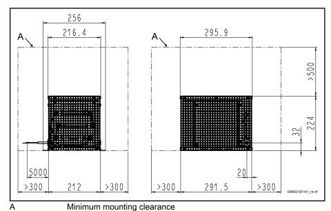
Fig.8-47: Dimensions (with Upright Mounting on the Floor)
