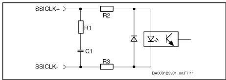
Fig.7-24: Differential Input Circuit (Block Diagram)
