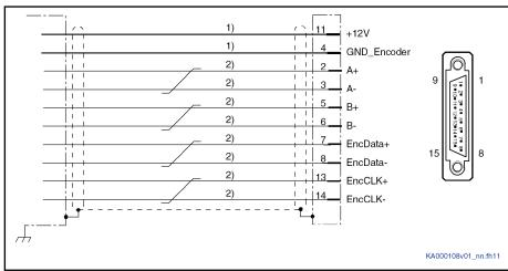
1) Line cross section ≥ 0.5 mm²; observe allowed encoder cable length
