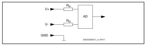
AD Analog/digital converter Fig.7-34: Analog Voltage Input
