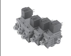
The 3/2 function Series 579 directional control valve with unique poppet design offers trouble free service. Polymer body allows a rugged and corrosion resistant valve. Dove tail design allows combining of valves easily without tools. Integrated pneumatic tube fittings save time and money.
