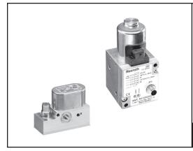
Direct acting poppet style, electro-pneumatic (E/P) pressure control valves with closed loop control. Use to change output pressure or force proportional with an electrical input. Compact ED02 version is only 30mm wide. Also in the GoTo program is the higher flow ED05 model.
