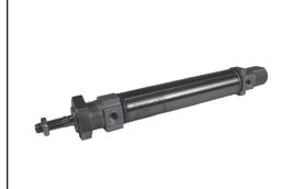
The Series MNI mini-ISO cylinder conforms to ISO 6432, ensuring interchangeability between manufacturers who conform to the same standard. With stainless steel rod and barrel, anodized aluminum end covers, brass piston and Buna-N seals, it provides a rugged construction ensuring years of trouble-free operation. Included in GoTo are bore sizes range from 12mm to 25mm, with strokes 10mm, 25mm, 50mm, 80mm, 100mm and 160mm. A comprehensive array of a mounts and rod accessories are available.
