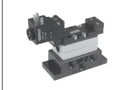
Series 581 directional control valves meet ISO 5599-1 and are interchangeable with many other manufacturers. The 581, in ISO sizes 1, 2 and 3 offers higher flow rates as compared other ISO valves within the same size. Unique spool and sleeve assembly is isolated from vibration and outside forces for long life. Construction allows field convertibility for internal or external pilot control. Valves come with CNOMO operators, coils to be ordered separately. Subbases also ordered separately.
