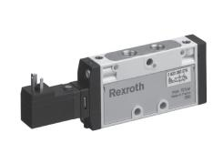
Compact pneumatic directional control valves with polymer body and metal threaded inserts. The GoTo program includes 1/8" (TC08) or 1/4" (TC15) valves with NPT and ISO-G porting as inline versions, and NPT only as manifold components for up to 12 stations.
