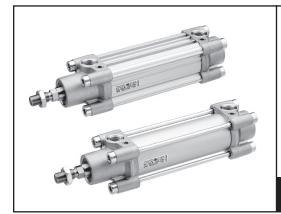
Series PRA and TRB double acting air cylinders have aluminum bodies providing a clean and robust design. The PRA is a profile (non-tie rod) version, the TRB has tie rods with a round tube. Ideal cushioning maximizes speed and load carrying capabilities. Interchangeable with many other manufacturers of ISO 15552 cylinders. Configure complete cylinders (from 32mm to 125mm bore sizes) online within limitations listed below.
