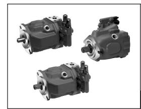
Variable displacement axial piston pump (A)A10V(S)O in swashplate design is available for open circuit applications. It can be used in both mobile and industrial applications. Flow is proportional to the drive speed and the displacement. By adjusting the position of the swashplate, it is possible to steplessly vary the flow. Multiple forms of pressure, flow or electrohydraulic controls are available.
