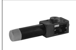
The valve type DR 6 DP is a direct operated pressure reducing valve in 3-way design, i.e. with pressure limitation of the secondary circuit.
