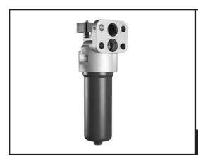
Manifold mounted filters are designed to be mounted directly on the pump outlet or control manifolds. They are installed upstream to protect open-loop and closed-loop control systems.
