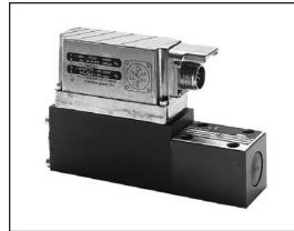
DBETBEX proportional pressure relief valves limit pressure for piloting applications requiring high performance. Pressure is directly controlled by changing the proportional solenoid position with on-board electronics (OBE).
