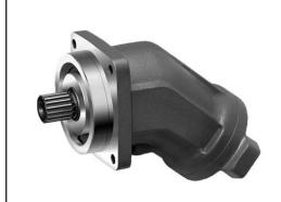
Fixed displacement motor (A)A2FM in axial tapered piston rotary group of bent-axis design is applicable for closed and open circuit applications. It can be used in both mobile and stationary applications. The output speed is dependent on the flow of the pump and the displacement of the motor. The output torque increases with the pressure differential between the high-pressure and the low-pressure side. The (A)A2FM motor has excellent starting torque efficiency.
