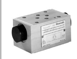
Models Z2SRK are pilot operated check valves in a sandwich plate design. They provide line contact closure in one or two actuator ports, even during idle periods. Piloted to open, utilizing a pressure signal from the opposite actuator port provides a self-contained function. The Z2SRK has a maximum operating pressure of 3000 PSI.
