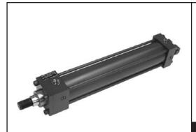
Rexroth offers you a well structured and systematically engineeredrange of hydraulic cylinders geared to your application requirements. Our CDT1/4 cylinders conform to NFPA standards regarding bore, rod, mounting, and length. Manufactured and assembled in the U.S.A., CDT1 cylinders are rated ro 1500 PSI and the CDT4 for 3000 PSI. A full array of bores and rod diameters cover the spectrum from 1" to 8".
