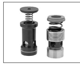
M-SR check valves are cartridge assemblies for use in manifold applications. Flow capacities of 8 GPM – 106 GPM over six cartridge sizes permit a broad application potential. Both the right angle version "KE" or straight through version "KD" feature guided poppets with varying biasing spring options. M-SR check valves can be secured in a manifold utilizing a BSP or SAE plug (pressure limits applicable). The cavity is a relatively straight bore, therefore complicated tooling is not required.
