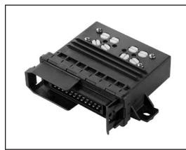
The analog amplifier activates up to two proportional solenoids. The specified control voltage is processed in the amplifier as an input command signal. The analog amplifier provides a regulated electric current as an output signal for actuation of proportional solenoids.
