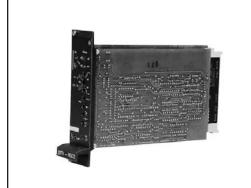
The VT-VRPA1 is suitable for controlling servo solenoid pilot operated two-stage valves. It has options for valve zero and gain. The ramps can be controlled by external voltage signals.
