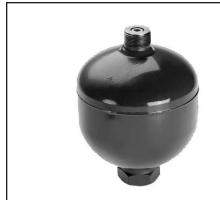
The HAD design is a hydro-pneumatic type accumulator that utilizes compressed nitrogen to supply fluid to the hydraulic system. The nitrogen and hydraulic fluid are separated by means of an elastomeric membrane. HAD units are the diaphragm welded non-repairable type that can be supplied in both non-rechargeable and chargeable versions.
