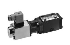
Model DRE6X proportional pressure reducing valves are pilot operated with a 3-way main stage. The pilot valve (pressure relief valve pilot stage) is supplied internally with a controlled flow of pilot oil. The valves are actuated by a proportional solenoid acting against a spring. The solenoid armature is cushioned to aid stability.
