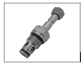
Solenoid-operated, 2-way / 2-position, normally closed, pilot operated, poppet-type, cartridge valve. When de-energized, flow is permitted across the check valve function from port 1 to 2, and blocks flow leak-free from port 2 to 1. When the coil is energized, the valve allows bi-directional flow between both ports.
