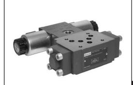
Valve type Z4WEH are directional spool valves with electrohydraulic actuation. They control the start and stop of a flow, and function as an emergency on–off isolating valve or on–off isolating/bypass valve, primarly used for servo/proportional systems.
