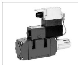
Pilot operated proportional directional valve type 4WRVE offers integral position feedback on both pilot and mainstage for dynamic response plus greater accuracy. On-board electronics (OBE) and 12-pin connectors permit power and command all to be accomplished on the valve. Underlapped main spools and high performance pilot permit the WRVE to be an excellent candidate into applications requiring closed loop control of pressure, force, and velocity.
