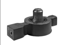
The valve type ZSF is a pilot operated check valve in sandwich plate design. It is used for the leakage-free isolation of pressurized working circuits (e.g. pressing cylinders). Due to its favorable flow characteristics and the low cracking pressure of the main poppet, it is particularly suitable on presses.
