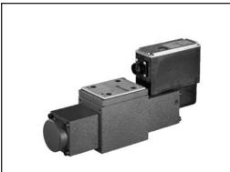
These 4/3 directional high-response valves are direct operated components. They are actuated by control solenoids. The solenoids are controlled by integrated control electronics (OBE).
