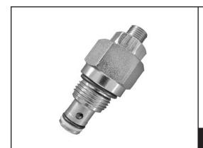
With flow from 2 to 1, the valve provides a fully adjustable orifice restriction. Free flow is permitted from 1 to 2, regardless of valve adjustment, by when pressure overcomes the spring bias of the valve's check function. STFU, compared to STVU, is suitable for applications requiring fine adjustments.
