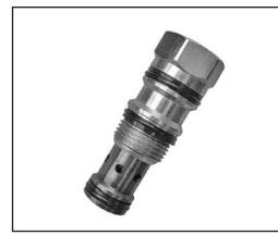
When pressure at 2 rises above the spring bias pressure, the poppet is pushed from its seat and flow is allowed from 2 to 1. The valve is normally closed (checked) from 1 to 2. When sufficient pilot pressure is present at port 3, the pilot piston acts to push the poppet from its seat and flow is allowed from 1 to 2. Precision machining and hardening processes allow virtually leak-free performance in the checked condition. Available with "manual override" option.
