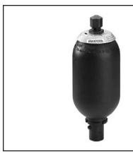
The HAB design is a hydro-pneumatic type accumulator with compressed nitrogen separated from hydraulic fluid by means of an elastomeric bladder. The current generation of bladder accumulators from Bosch Rexroth carries the HAB-5X designation. The HAB product line is available in many different configurations needed to meet the stringent demands of today's market.
