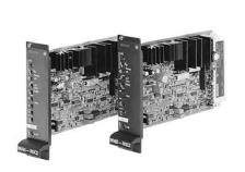
The VT-VRPA2-5.../RTP/ is suitable for controlling direct operated 4WRP valves. It offers both zero and maximum adjustments for both solenoids. Ramp times are set by potentiometer adjustments for both acceleration and deceleration.
