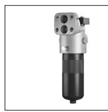
Manifold mounted filters are designed to be mounted directly on the pump outlet or control manifolds. They are installed upstream to protect open-loop and closed-loop control systems.
