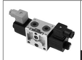
The sandwich plate design directional valve elements L8\_10... are compact direct operated solenoid valves which control the start, the stop and the direction of the oil flow.
