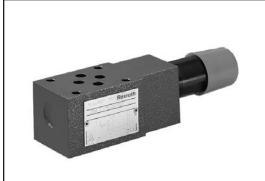
Pressure relief valve types ZDB(K) und Z2DB are pilot sandwich type pressure controls. ZDB versions offer single port pressure control, while Z2DB models offer dual port pressure control. Z2DB models can be configured as either port relief or cross port relief. The ZDB program offers multiple spring options.
