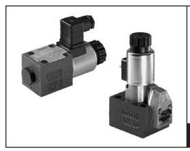
Directional control valves, model SED and SEW, are direct (SED) or lever (SEW) actuated directional poppet valves with solenoid actuation. They control the start, stop, and direction of fluid flow. Poppet valves, or seat valves, provide a line contact closure for applications where spool valve leakage or silting is not desirable.
