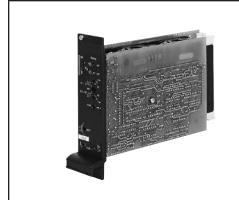
The VT-VRPA1-527 controls throttle cartridge valves FESX with
