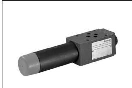
Models ZDR are 3-way direct operated pressure reducing-relieving valves. They maintain a "reduced" pressure in a branch circuit and permit "relieving" pressure spike occurrences in the reduced branch circuit. Options for pressure ranges and operator adjustment options are within the scope of the modular reducing valve portfolio.
