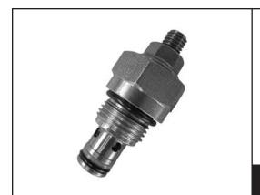
Flow is blocked from 1 to 2 until pressure increases to meet the selected valve setting, lifting the poppet from its seat and allowing relief flow through port 2 to tank. Pressure at port 2 is additive to the relief setting of the valve. The unique Bosch Rexroth Oil Control poppet design provides enhanced stability at all flows and pressures.
