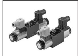
Directional valves type WE are solenoid operated directional spool valves. They control the start, stop, and direction of a flow. These directional valves basically consist of housing; one or two solenoids; control spool; and no, one, or two return springs. A full array of spools are possible with variations in voltage and electrical connection, all within the program. Flow and pressure rates from 4000 PSI to 5000 PSI and 21 GPM to 32 GPM cover a wide range of applications.
