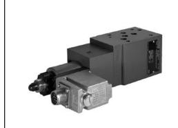
Valve of type ZDREE are pilot operated pressure reducing valves of sandwich plate design in 3-way variant, i.e. with pressure limitation of the actuator pressure. They are used for reducing a system pressure.
