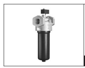
Line filters are used in hydraulic systems for separating solid materials from the hydraulic fluids and lubricating oils. They are intended for installation into pipelines.
