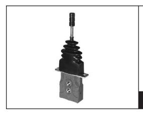
Hydraulic pilot control units of the type 2TH6 operate on the basis of direct operated pressure reducing valves. Pressure in the relevent control port is proportional to the stroke of the control lever. This pressure control as a function of the control lever position and the characteristics of the control spring enables the proportional hydraulic control of directional valves and high response control valves for hydraulic pumps and motors.
