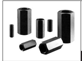
S model check valves are direct operated, line contact seat, guided poppet check valves. Guided poppets vs a "ball" provide more stable operation, more assurance for a line contact seat, and reductions in flow noise. The line contact seat is an interference fit where the seat areas are at slight differential angles to permit a true line contact seat vs a matched mating surface.
