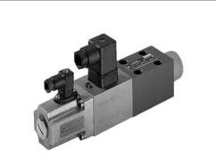
The VT-DFP-A-2X/G24K0/0/V is the pilot control valve for the SYDFE1 system. In conjunction with amplifier VT5041, it controls the swashplate angle of the pump in either closed loop pressure or flow control. This valve is to be considered a part and not a complete control.
