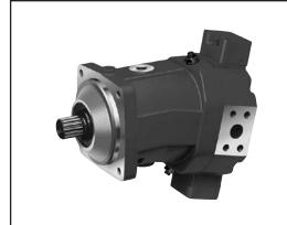
Variable displacement motor (A)A6VM in axial tapered piston rotary group of bent-axis design is available for open and closed circuit applications. It can be used in both mobile and industrial applications. The output speed is dependent on the flow of the pump and the displacement of the motor. The output torque increases with the pressure differential between the high-pressure and low-pressure side and with increasing displacement.
