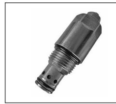
When pressure at 2 rises above the spring bias pressure, the poppet is pushed from its seat and flow is allowed from 2 to 1. The valve is normally closed (checked) from 1 to 2. When sufficient pilot pressure is present at port 3, the pilot piston acts to push the poppet from its seat and flow is allowed from 1 to 2. Precision machining and hardening processes allow virtually leak-free performance in the checked condition. Available with "manual override" option.
