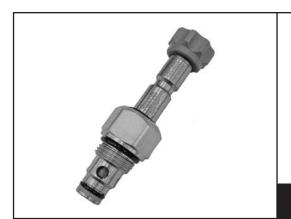
Solenoid-operated, 2-way / 2-position, normally closed, pilot operated, poppet-type, cartridge valve. When de-energized, flow is permitted across the check valve function from port 1 to 2, and blocks flow leak-free from port 2 to 1. When the coil is energized, the valve allows bi-directional flow between both ports.
