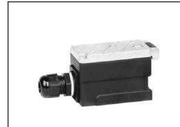
The plug amplifier is employed for actuating proportional valves without position control. It is plugged directly onto square solenoid valves. User can adjust ramp time, dither, and minimum and maximum output current.
