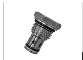
When pressure at 1 rises above the spring bias pressure, the poppet is lifted and flow allowed from 1 to 2. The valve is closed (checked) from 2 to 1. Precision machining and hardening processes allow virtually leak-free performance in the checked condition.
