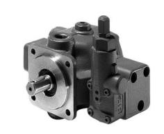
The PV7 is a variable displacement vane pump used quite extensively for low to mid-pressure applications for numerous market segments such as machine tool and packaging industries. The PV7 pump utilizes a journal bearing design and pivoting control pistons to provide a low noise and durable product for the industrial hydraulic market.
