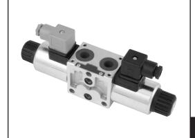
The sandwich plate design directional valve elements L8080... are compact direct operated proportional solenoid valves which control the start, the stop, the direction and the quantity of the oil flow.
