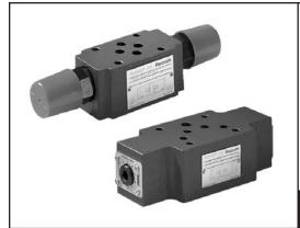
Flow control valves, Model Z2FS(K), are double throttle/check sandwich type valves. They restrict flow to or from actuator ports (A & B) of a directional valve. Two throttle/check valves, symmetrically arranged in the housing, restrict flow with adjustable throttles in one direction while providing free flow in the opposite direction.
