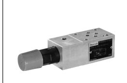
Models ZDRK are 3-way direct operated pressure reducing-relieving valves. They maintain a "reduced" pressure in a branch circuit and permit "relieving" pressure spike occurrences in the reduced branch circuit. Options for pressure ranges and operator adjustment options are within the scope of the modular reducing valve portfolio.
