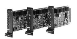
The VT-VRPA1-537-1X/V0/PV-RTP is used to control direct operated pressure control valves DBETBX. It has both zero and maximum adjustments to optimize the pressure range for the hydraulic circuit. Ramp times are controlled by potentiometer adjustment.
