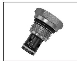
When pressure at 1 rises above the spring bias pressure, the poppet is lifted and flow allowed from 1 to 2. The valve is closed (checked) from 2 to 1. Precision machining and hardening processes allow virtually leak-free performance in the checked condition.
