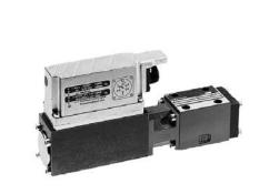
DREBE6 is a pilot operated pressure reducing/relieving valve for high performance applications. Pressure in port A is controlled by a proportional solenoid using position feedback with on-board electronics (OBE).
