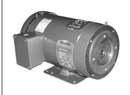
Close-Coupled Motors are NEMA frame, female shaft to accomodate SAE A (2-bolt flange 82-2 A SAE J744) pumps. Can be run at 60 HZ/1750 RPM/208-230/460 V or 50 Hz/1425 RPM/190-208/380-416 V.
