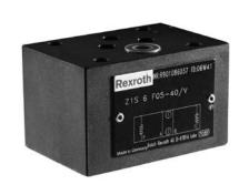
Valve type Z1S is a direct operated check valve of sandwich plate design. They provide line contact closure in one direction and allows free flow in the opposite direction. The check function can be in one of several ports, or dual ports. The check function orientation can also be defined by model coding.
