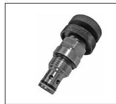
With flow from 2 to 1, the valve provides a fully adjustable orifice restriction. Free flow is permitted from 1 to 2, regardless of valve adjustment, by when pressure overcomes the spring bias of the valve's check function.
