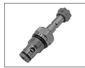
Solenoid-operated, 2-way / 2-position, normally open, pilot operated, poppet-type, cartridge valve. When de-energized, the valve allows bi-directional flow between both ports. When the coil is energized, flow is permitted across the check valve function from port 1 to 2, and blocks flow leak-free from port 2 to 1.
