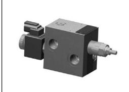
The inlet elements TA-05-\_ are employed to connect the external P and T lines to the P and T channels inside the ED elements of the Directional Valve Assembly. They incorporate a pressure relief cartridge which limits the primary pressure in the P line. The relief setting can be checked through the Test Point port G.
