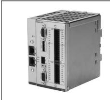
The VT-HACD-3-2X closed-loop control electronics is a module that is installed on a top hat rail. A microcontroller controls the entire process, makes adjustments, establishes links and realizes the closed control loops. Data for configuration, command values and parameters are stored in a FLASH in a non-volatile form.
