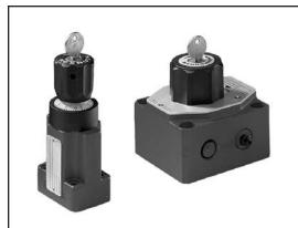
Pressure compensated flow controls Model 2FRM are two-way restrictive-style flow regulators. They accurately control flow, independent of changes in fluid viscosity or pressure drop across the valve. This valve maintains a constant actuator speed independent of changes in load induced pressure. Sharp edged throttle openings reduce the influence of flow variations from temperature change.
