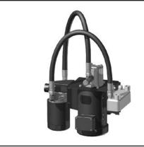
The MFC3 is a compact off-line filtration/ cooling package, which provides numerous mounting and configuration options. The design allows for multiple selections of AC motors, pumps, filter elements, and auxiliary components. The modular design concept permits field upgrades concerning oil flow, filtration, or configuration with minimal labor and cost.
