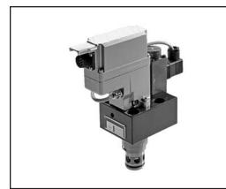
Model FESXE proportional throttle valves are pilot operated and in "cartridge" design. This results in their compact form despite high flow rates. The position of the main spool is closed-loop controlled by the on-board electronics (OBE).
