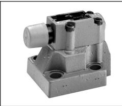
Pressure control valves of type DB are pilot operated pressure relief valves. They are used for the limitation of the operating pressure. Pressure relief valves basically consist of a main valve with main spool insert and pilot valve with pressure adjustment element.
