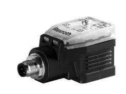
The plug-in amplifier is suitable for mounting onto a valve connection base according to EN 175301-803. By turning the plug insert and the electronics in the housing, the plug-in amplifier can be mounted on the solenoid in 90° increments. user can adjust ramp time, maximum current, and bias current.
