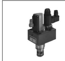
Model FESX proportional throttle valves are pilot operated and in "cartridge" design. This results in their compact form despite high flow rates. The electronics, which take the form of an external valve amplifier in Europe card format, trigger the solenoid of the pilot valve and thus control the position of the main stage. Hysteresis is <0/2% and a position accuracy of >0.5% is achieved.
