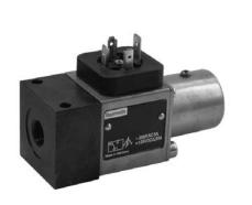
Hydro-electric pressure switches of model HED 8 are piston-type pressure switches used to monitor a pressure value in a circuit. As a pressure value is achieved (rising or falling), the HED micro-switch changes state, which can be used as an indicator for the next sequential operation or shutdown. The HED microswitch is not a current carrying device; it is an actuator/sensor.
