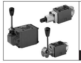
Directional valves type WMM are lever operated directional spool valves. They control the start, stop, and direction of a flow. These directional valves basically consist of housing; lever; control spool; return springs. A full array of spools are possible with variations for detented operation on both 2-position or 3-position functions. Flow and pressure rates from 4000 PSI to 5000 PSI and 16 GPM to 32 GPM cover a wide range of applications.
