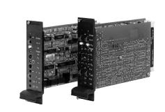
The p/Q amplifier is comprised of a base card with front panel containing the valve amplifier for 4WRPH6 with closed loop pressure controller. When used with the appropriate servo solenoid valves and pressure sensors, this unit can be employed for controlling flow and pressure in a closed-loop control circuit. The input parameters are the setpoints for pressure p and flow Q.
