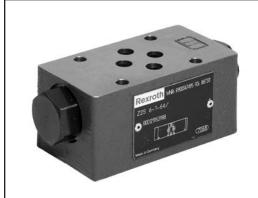
Models Z2S are pilot operated check valves in a sandwich plate design. They provide line contact closure in one or two actuator ports, even during idle periods. Piloted to open, utilizing a pressure signal from the opposite actuator port provides a self-contained function.
