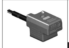
The VT-SSBA1 switching amplifier is directly mounted on the valve's K4 connector. It is supplied with 24 V direct voltage. As a fast switching amplifier, the VT-SSBA1 considerably reduces the switching time of standard directional valves in connection with 12 V solenoid coils. As a power reducer, the switching amplifier considerably reduces the holding current when using 24 V standard directional valves.
