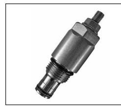
Flow is blocked from 1 to 2 until pressure increases to meet the selected valve setting, lifting the poppet from its seat and allowing relief flow through port 2 to tank. Pressure at port 2 is additive to the relief setting of the valve. The unique Bosch Rexroth Oil Control poppet design provides enhanced stability at all flows and pressures.
