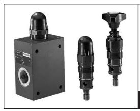
The DBD pressure relief valves are direct operated type relief valves. They are used to limit the pressure in a hydraulic system. DBD type relief valves offer line contact sealing for minimal leakage at closure and a full array of pressure capacities are available.
