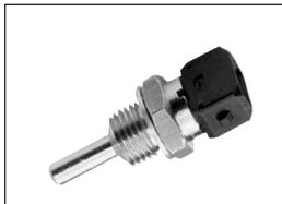
The sensor element consists of a PTC nickel-thin-film resistor, vacuummetalized onto a ceramic base. It enables the measurement of pressurized fluid temperatures of coolants, hydraulic oil or motor oil in vehicles. Its resistance increases virtually linearly with increases in temperature.
