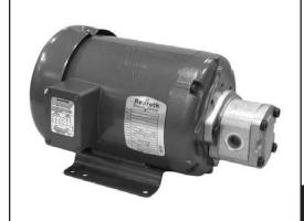
Close-Coupled Motor Pump Groups type MPGB-AZP come fully assembled from our factory. Pumps are external gear type, standard industrial keyed shaft. Motors are NEMA frame, femal shaft, and can be run at 60 Hz/1750 RPM/208–230/460 V or 50 Hz/1425 RPM/190–208/380–416 V.
