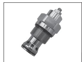
Flow is blocked from 1 to 2 until pressure increases to meet the selected valve setting, lifting the conical, pilot-stage poppet from its seat. This action exhausts oil above the main-stage piston (spool type), allowing it to shift and provide relief flow through 2 to tank. Pressure at 2 is additive to the relief setting of the valve. Pilot operation is protected from contamination by a filter screen at the bottom of the main piston.
